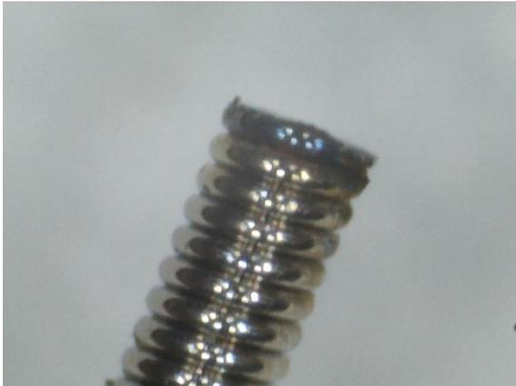
*Figure 5: Laser cut medical coil*
