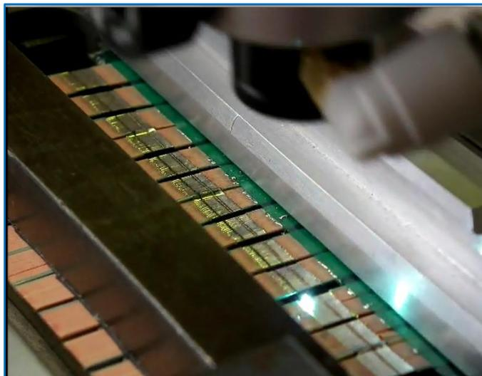
*Figure 4: Micro-coax ribbons in the process of being laser scribed on a Gemini-2*
