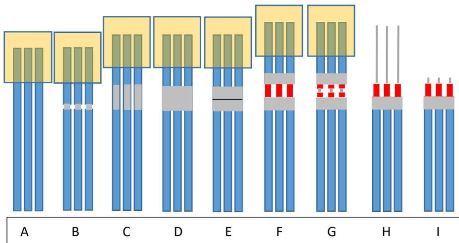
Figure 3: Laser Stripping Process with Soldered Scribing
