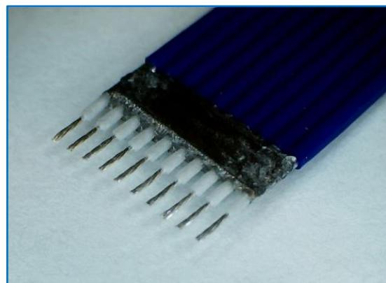
Figure 2: 42 AWG micro-coax ribbon – laser stripped
