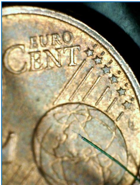
Figure 1: 50 AWG micro-coax – laser stripped
