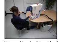
The Mercury-4 bench unit contains the laser and optics, whilst the power supplies are located with the fume extractor unit under the bench linked by an umbilical. Plenty of room on bench for hand tools, wires, finished goods, etc.
