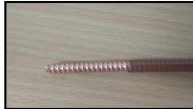
*Coroplast cable cleanly stripped using the Mercury-5 laser stripper*
