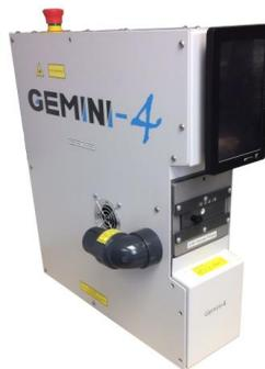
*A key factor in the design of the Gemini-4 has been to minimize the machine footprint on the operator's bench and set the wire load height at an ergonomic level when used from a sitting position. The small bench unit does not dominate the workspace allowing it to be used from a sitting position, with plenty of room for hand tools, wire and finished goods etc.*
