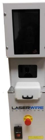
*The Mercury-4E bench unit contains the laser and optics, whilst the power supplies are located with the fume extractor unit under the bench linked by an umbilical. Plenty of room on bench for hand tools, wires, finished goods, etc.*
