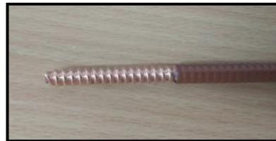
*Coroplast cable cleanly stripped using the Mercury-5 laser stripper*
